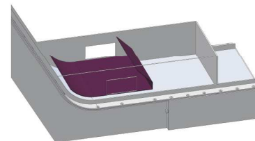
p.m. slide conveyor with funnel for filtration of fluids
